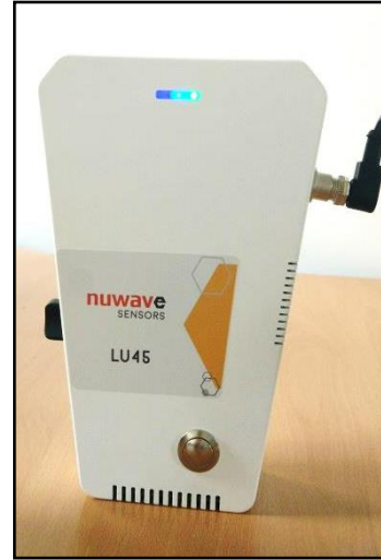
2. Push button, turning the light to blue with a flashing green
